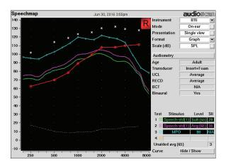
Or, compare predicted versus measured output/gain at specific frequencies. For example, in the image below, you see that predicted aided output for a 65 dB input at 2000 Hz is within 1 dB of the response obtained in the ear (though deviations within +/- 3 dB are acceptable).
